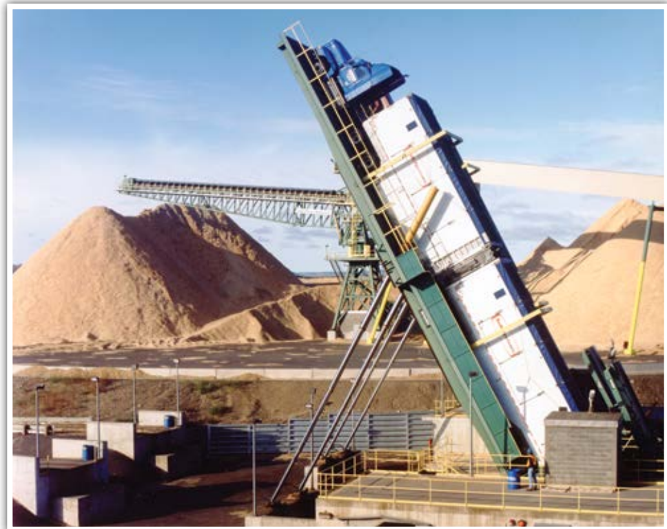
Trimac Bulk Systems woodchip B-Train on the tipper.
