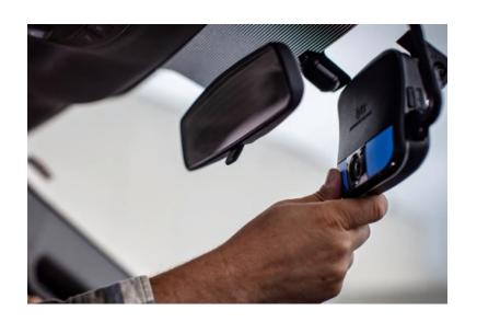
All company-owned and owner-operated vehicles are also equipped with Lytx Drive Cams, an intelligent video telematics device that uses machine learning and artificial intelligence to monitor external driving environments. The data collected by the Lytx Drive Cam is automatically uploaded into our safety portal, where our dedicated safety team analyzes driver behaviour and identifies potential risks.
